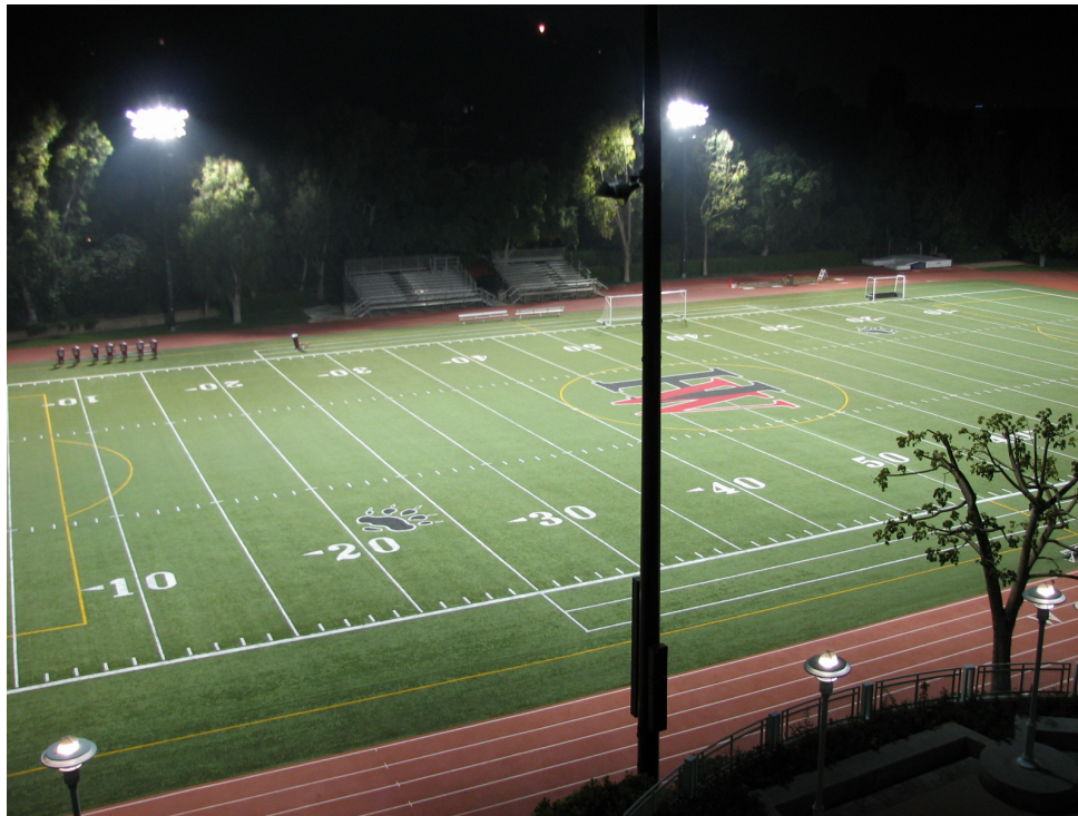
Figure 3.1-28 Night Lighting of Ted Slavin Field and Track Illustrating Precise Targeting of Lighting and Limited Spillover Lighting
